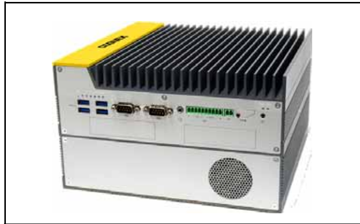
Figure 3-4: Scan Tunnel RTM Computer
