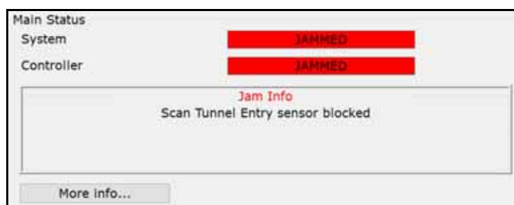
Figure 4-16: Sensor Blocked Jam
