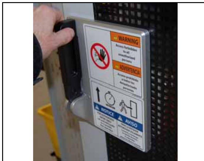
Figure 2-18: Door Interlock Detail
