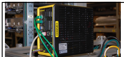
Figure 3-4: Scan Tunnel RTM Computer
