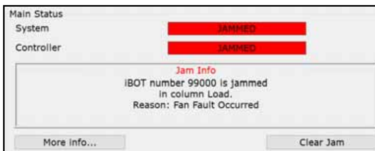
Figure 4-17: Fan Failure Jam
