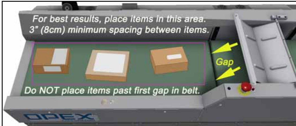
Figure 4-30: Conveyor "Drop Zone"
