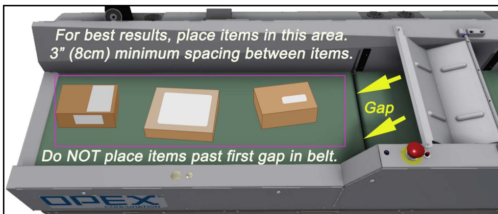
Figure 4-30: Conveyor "Drop Zone"
