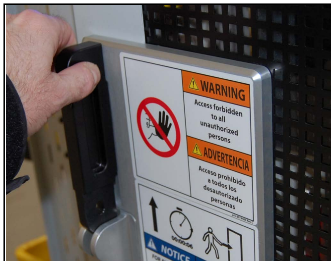
Figure 2-18: Door Interlock Detail
