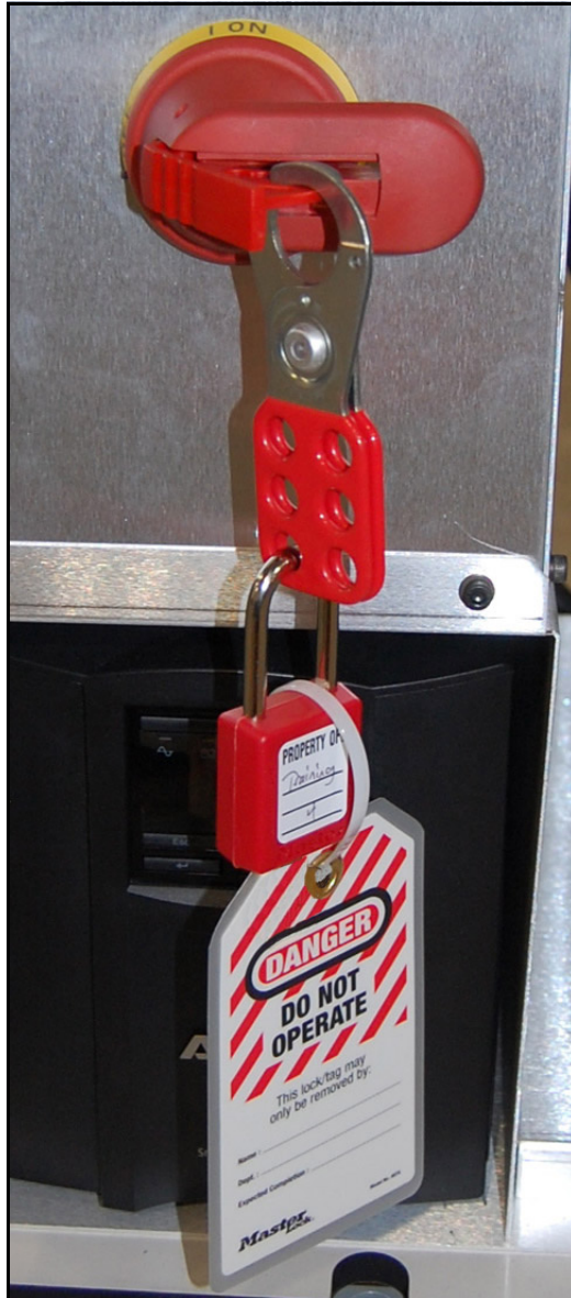
Figure 2-15: Lockout Tab with Hasp, Padlock and Tag
