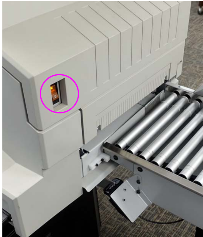
Figure 3-2: Falcon main power switch
