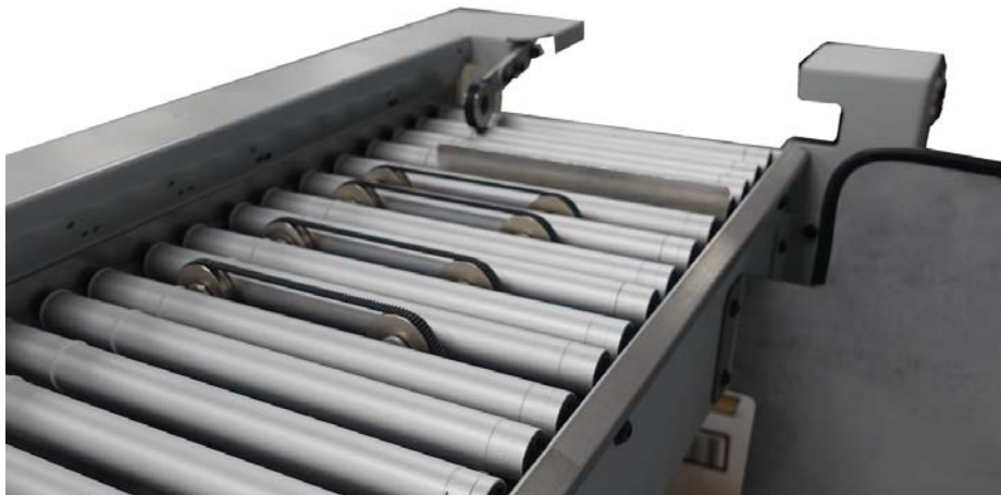
Gate Assembly for Bin 3 engaged
