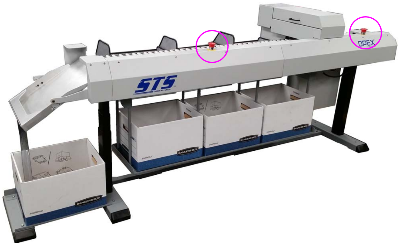
Figure 1-2: STS E-Stop locations
