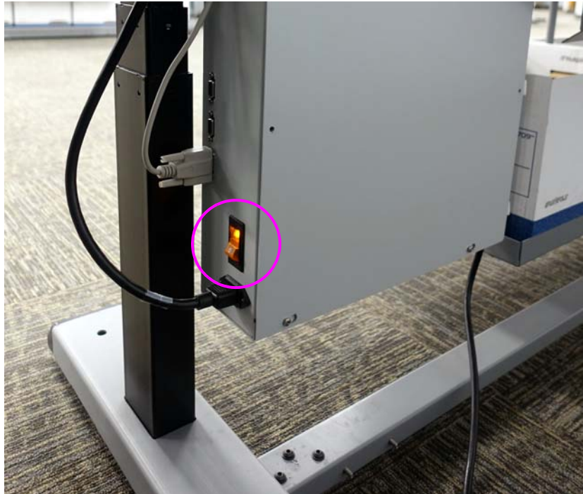
Figure 3-1: STS power switch
