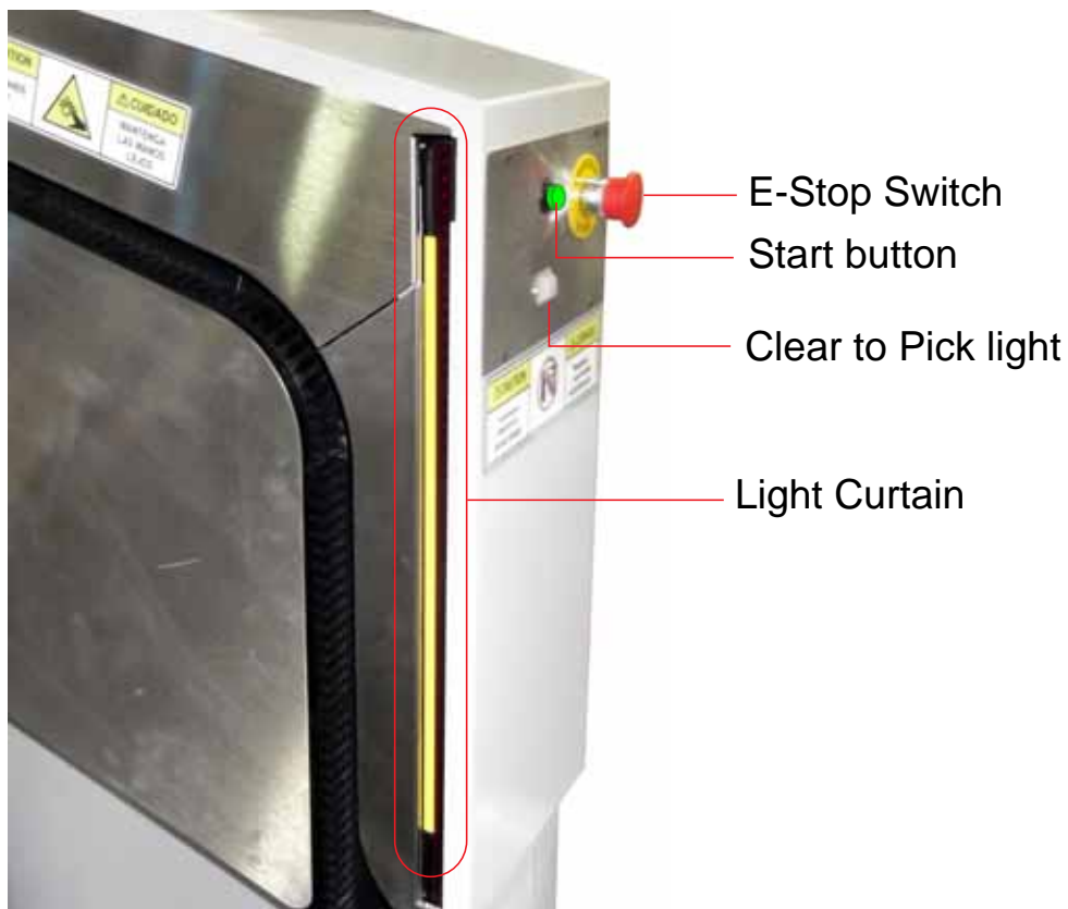
Figure 2: E-stop and interlock locations
