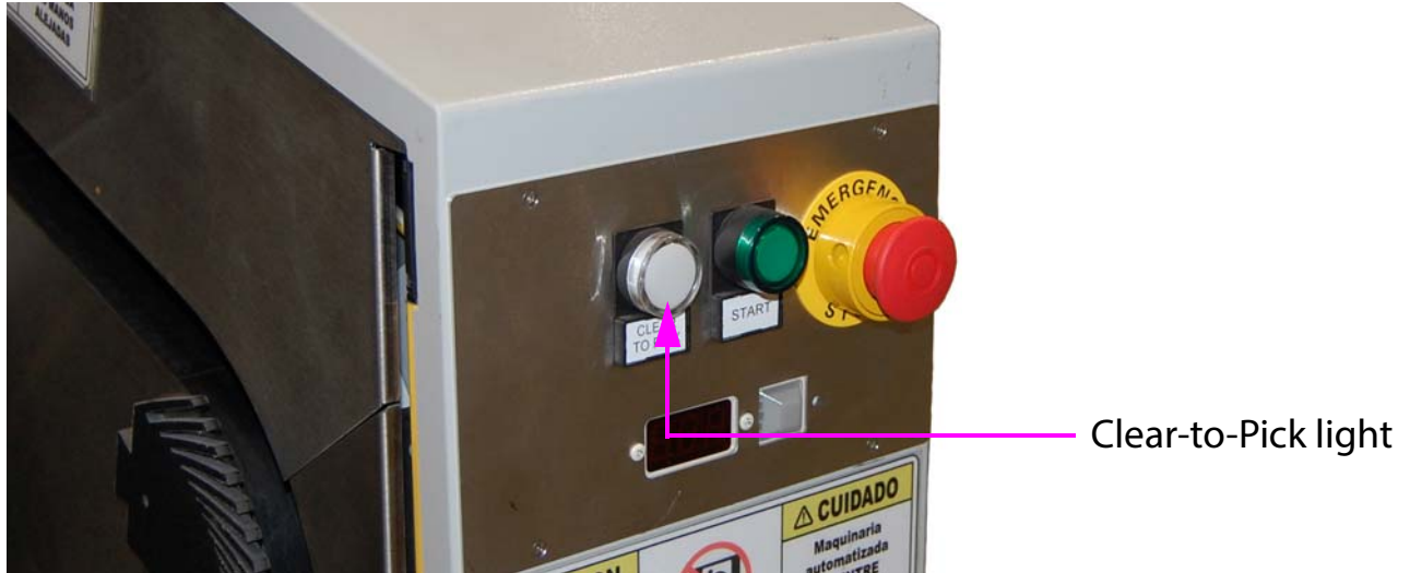
Figure 12: Pick station Clear-to-Pick indicator light
