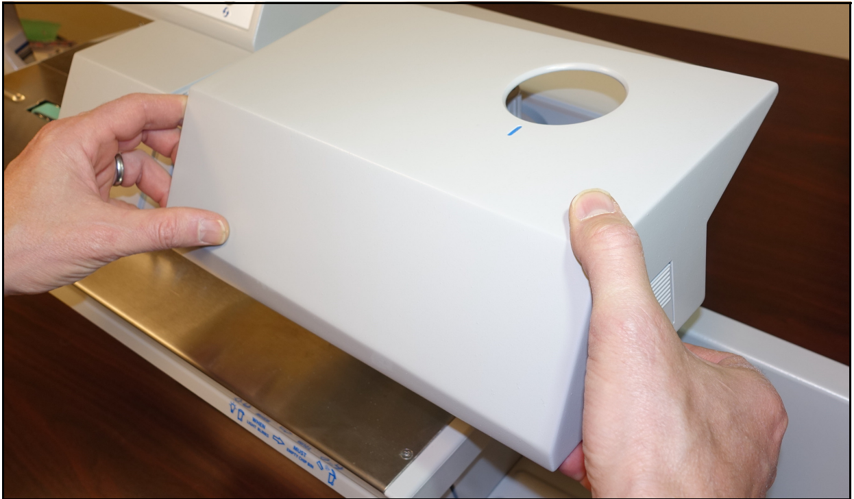
Figure 4-14: Lifting the Nip arm cover
