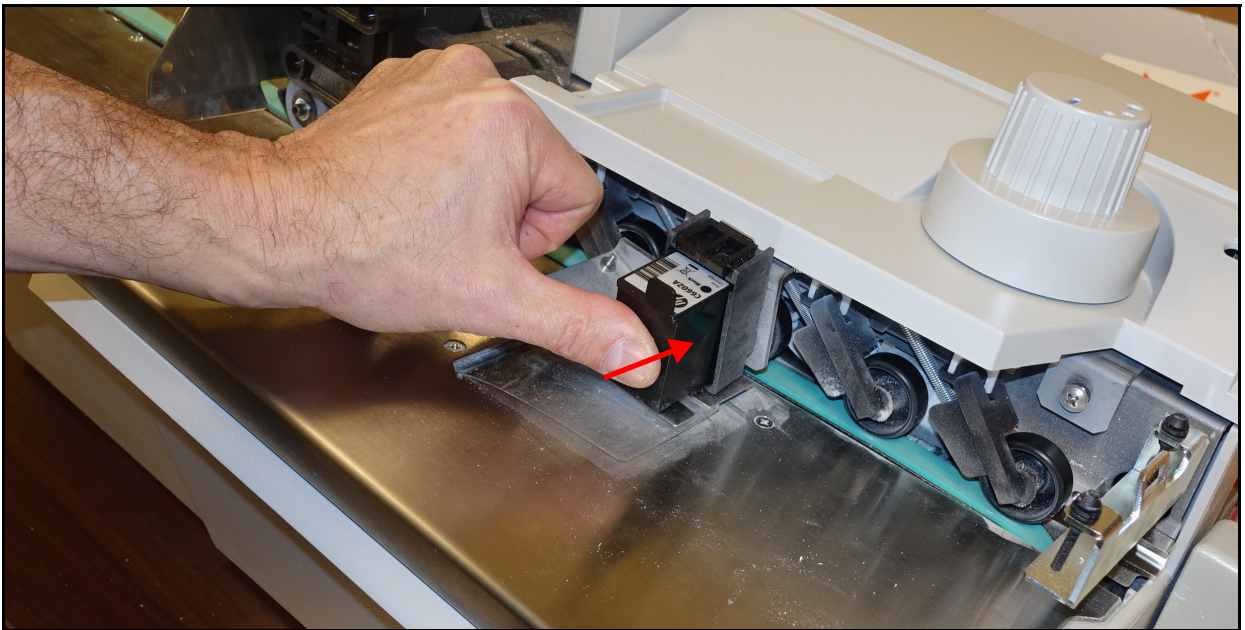
Figure 4-18: Replacing the printer cartridge
