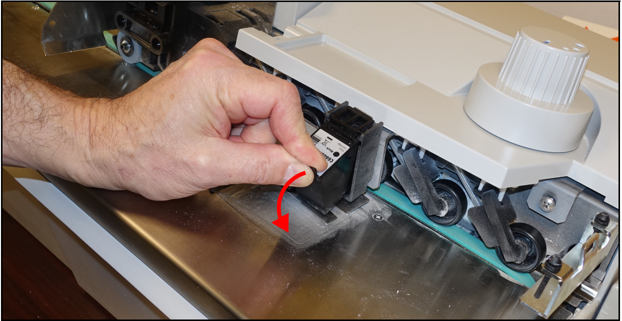
Figure 4-17: Removing the print cartridge
