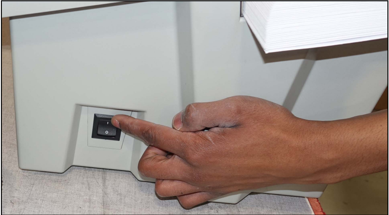
Figure 4-6: AC power switch
