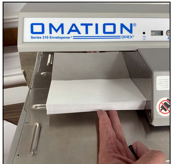
Figure 4-7: Loading the Envelope Feed Hopper
