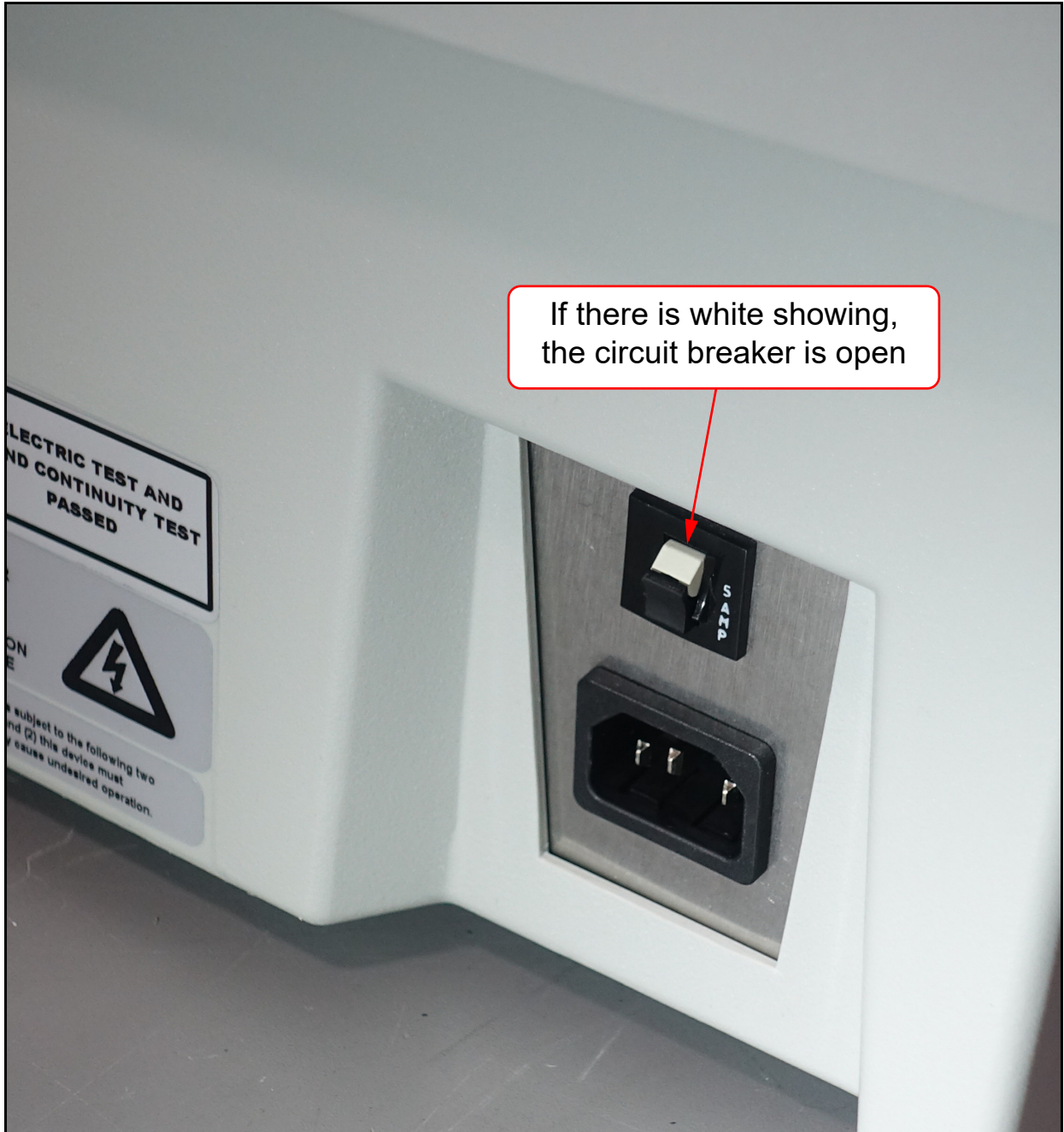
Figure 4-15: Open circuit breaker
