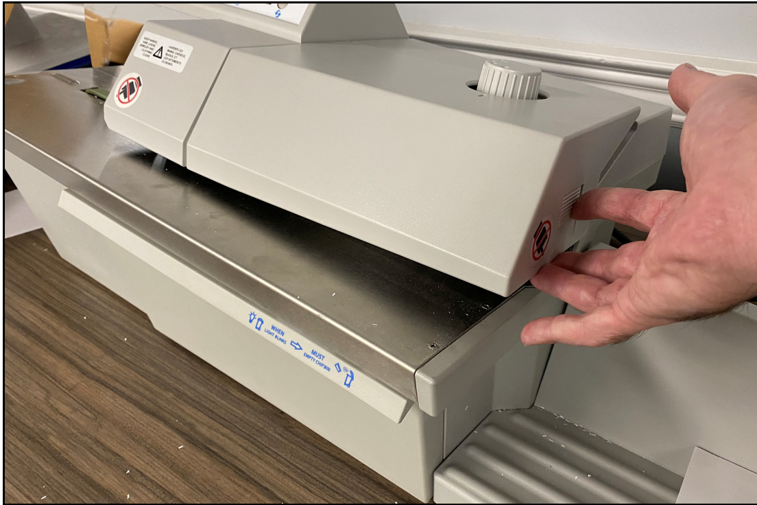
Figure 2-8: Top cover removal interlock triggering
