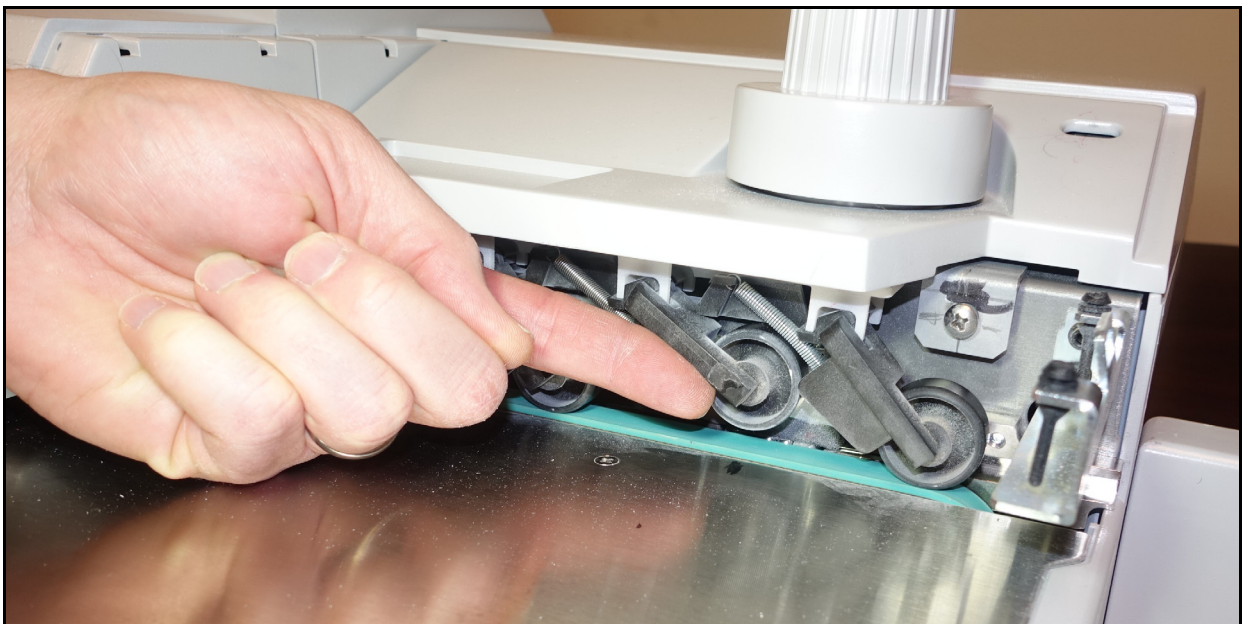
Figure 4-12: Cleaning under the nip wheels
