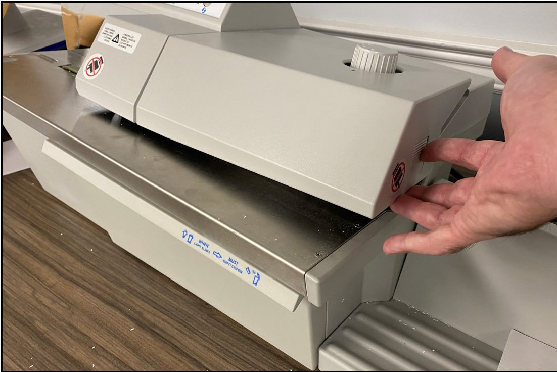
Figure 2-8: Top cover removal interlock triggering
