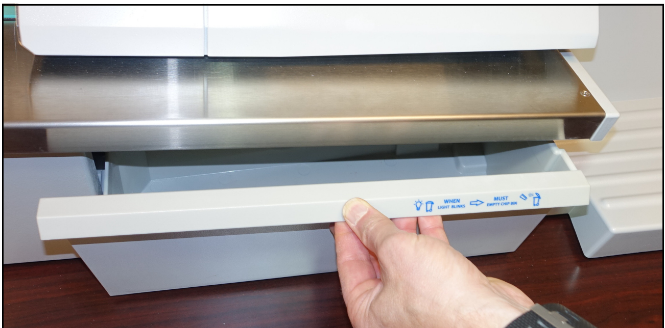
Figure 2-9: Bin tray removal interlock triggering
