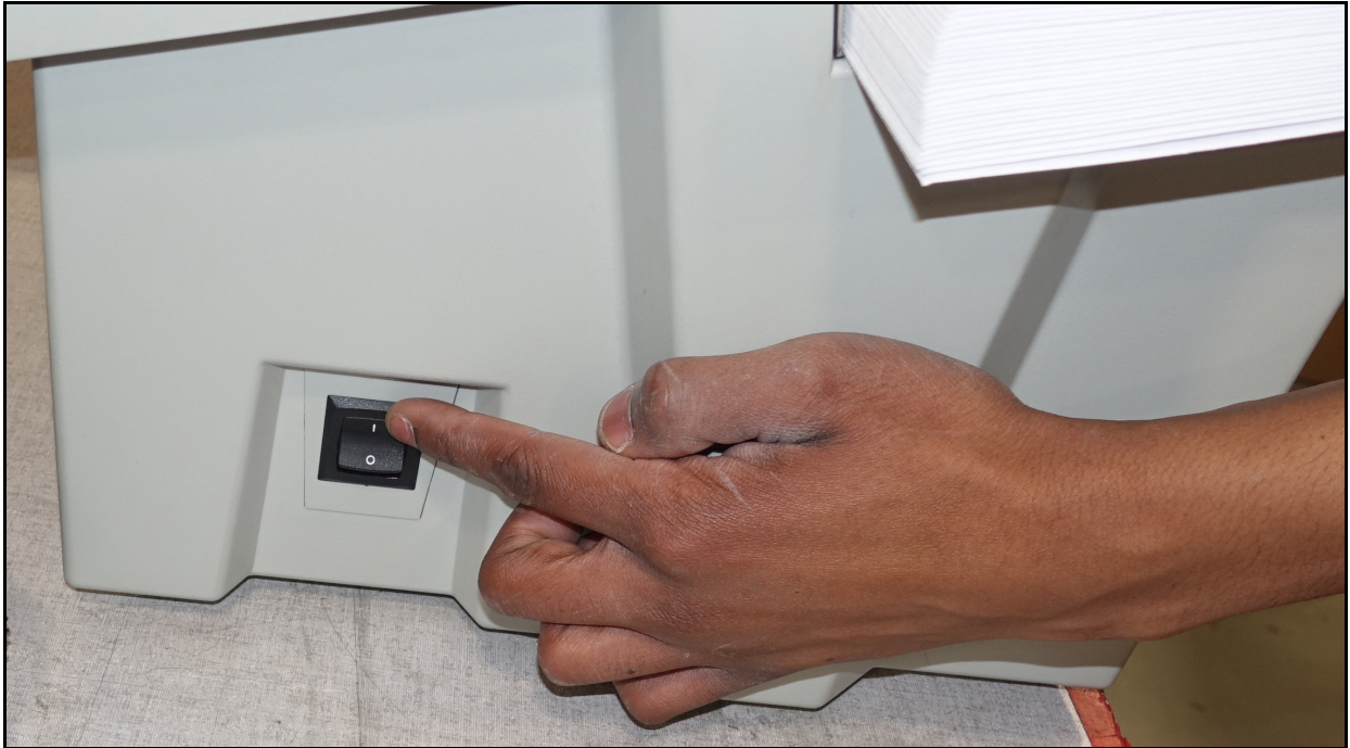
Figure 4-6: AC power switch
