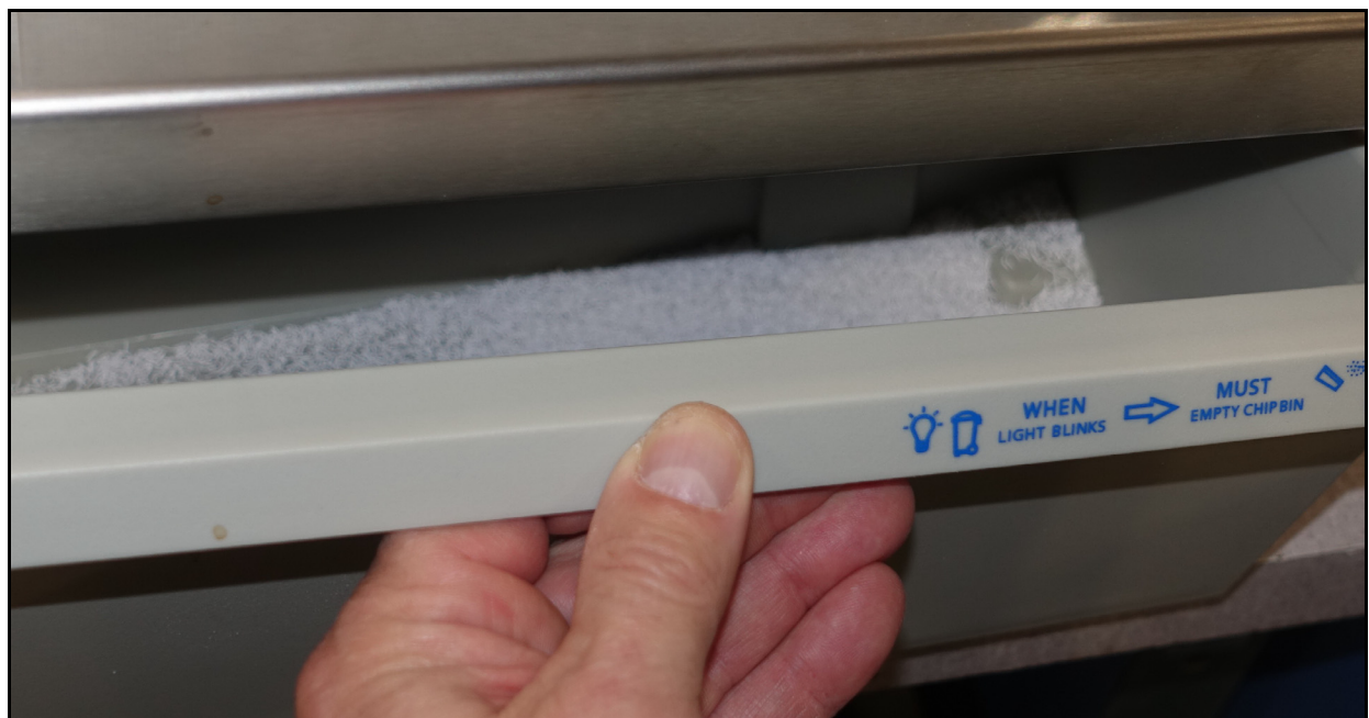
Figure 4-3: Opening the Chip Bin tray
