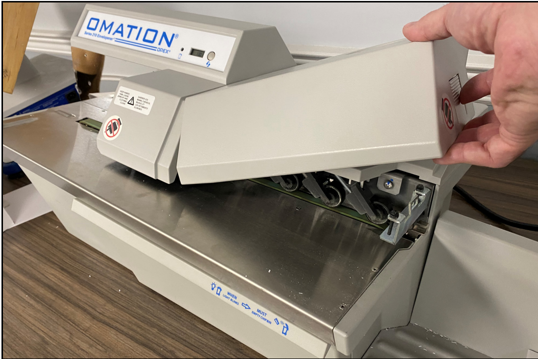
Figure 4-11: Lifting the Nip arm cover
