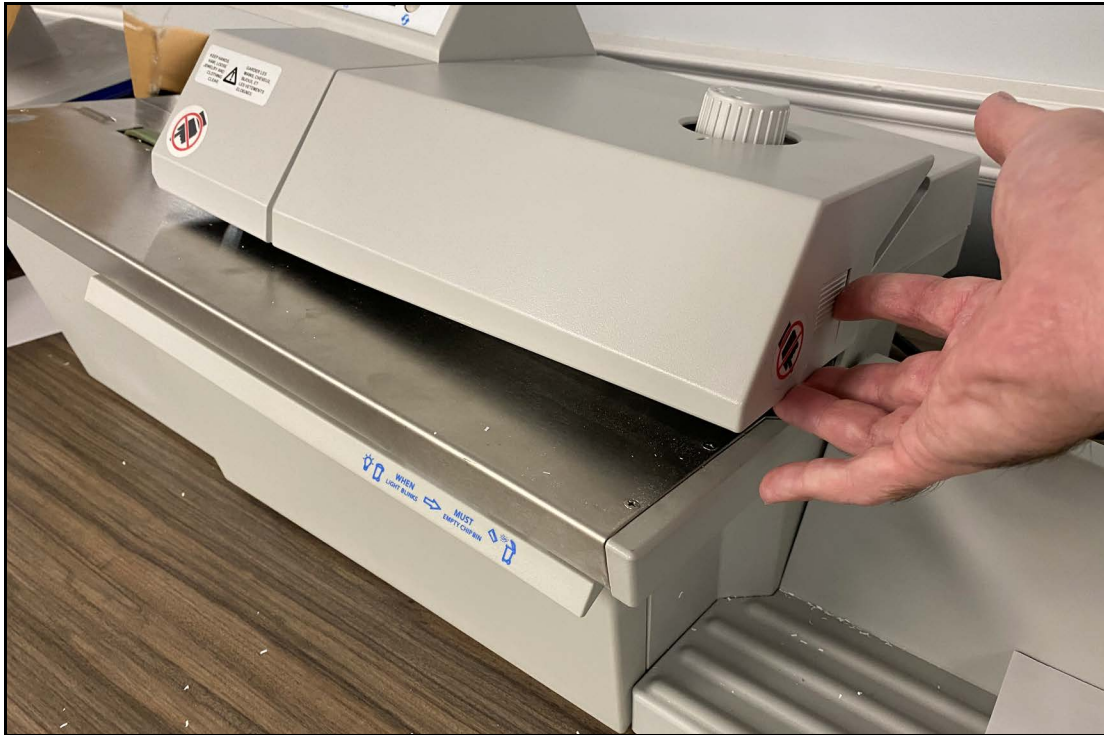
Figure 1-1: Top cover removal interlock triggering
