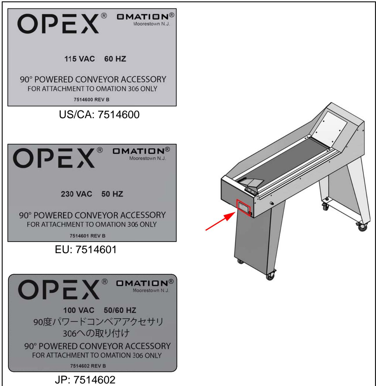
**Figure 2-10: Powered Conveyor Ratings label**
