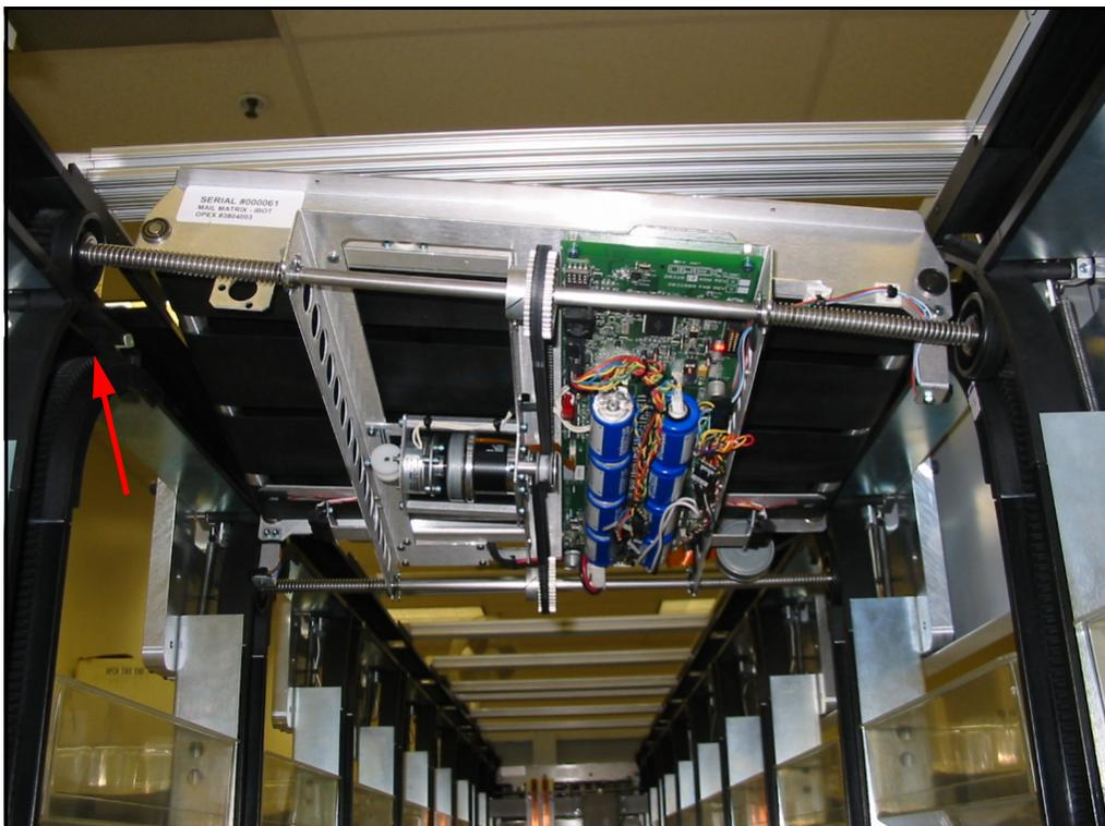
**Figure 135: Wheel traveling the wrong path after gate misfire**
