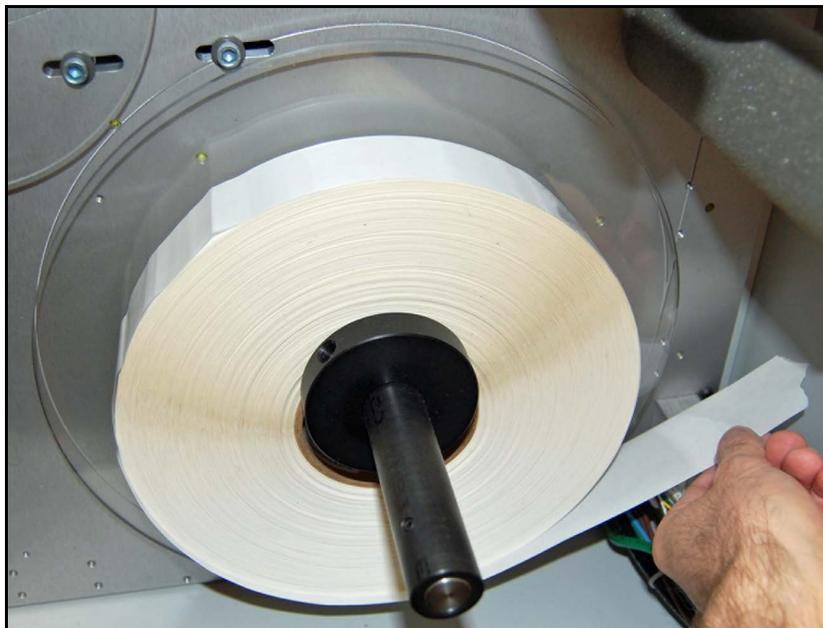
**Figure 102: Labels feed under and to the right**
