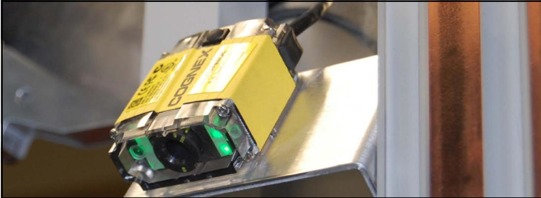
**Figure 87: Barcode verifier scanner**
