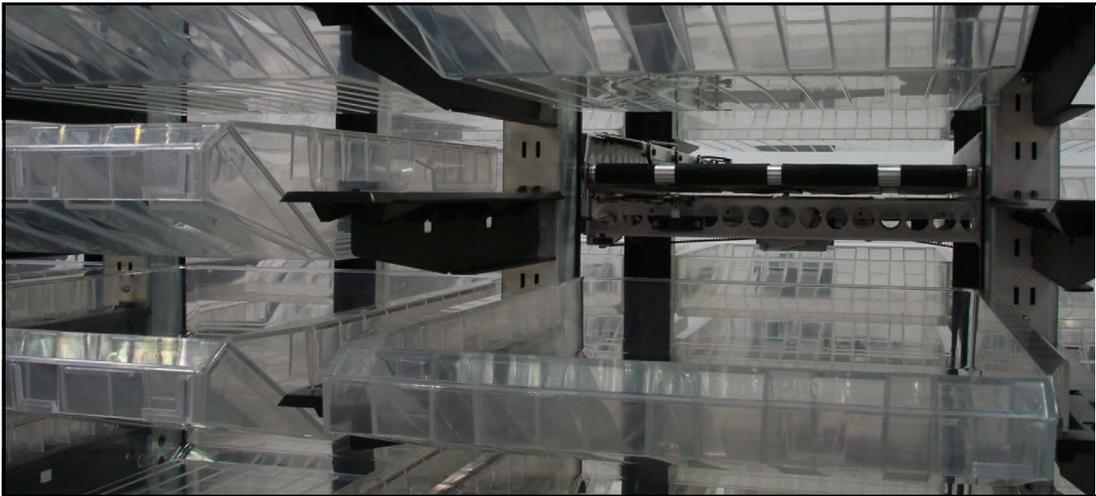
**Figure 64: iBOT stuck in a delivery column**
