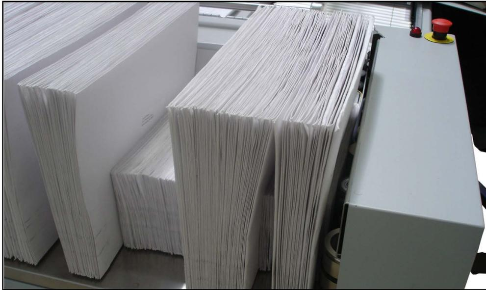
**Figure 54: Envelope feeder jam**
