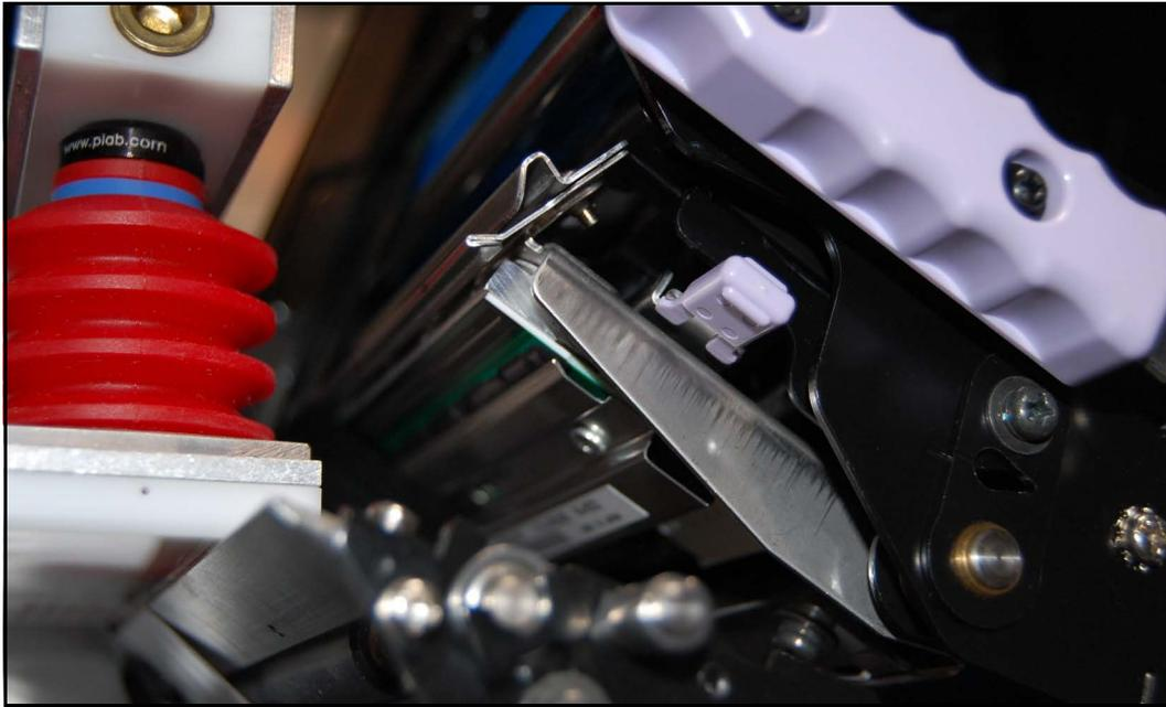
**Figure 115: New print head in place**
