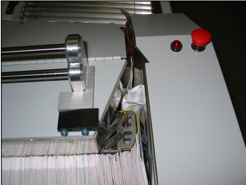
*Figure 132: Mail jamming the feeding mechanism*
