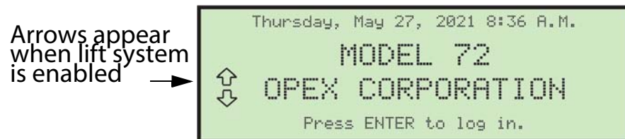
Figure 6-2: Lift system enabled
