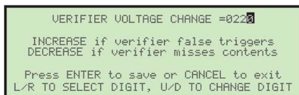
Figure 5-30: Verifier voltage change screen
