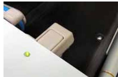
**IDAssist indicator** The blue IDAssist indicator LED will light up when running a job that includes IDAssist. Also, when the operator triggers IDAssist the LED will go out briefly, indicating to the operator that IDAssist has been activated. For more on using IDAssist, see “ID Assist” on page 67.
