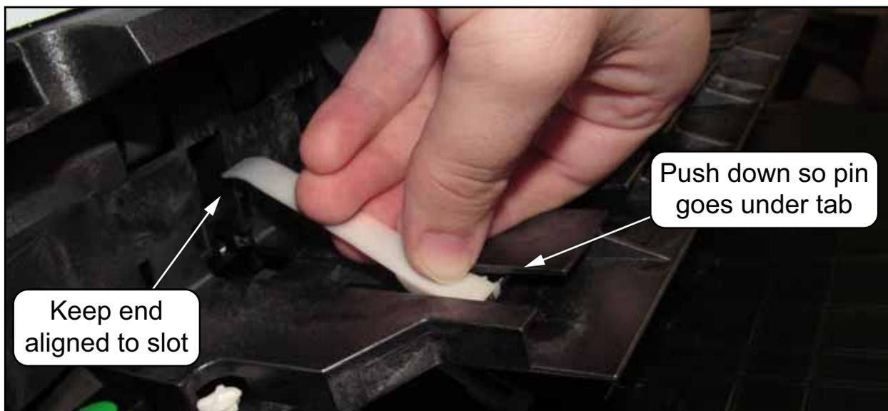
**Note:** On production machines, the stacker fingers are black. The white stacker finger shown above was used to provide better contrast in the photo.
