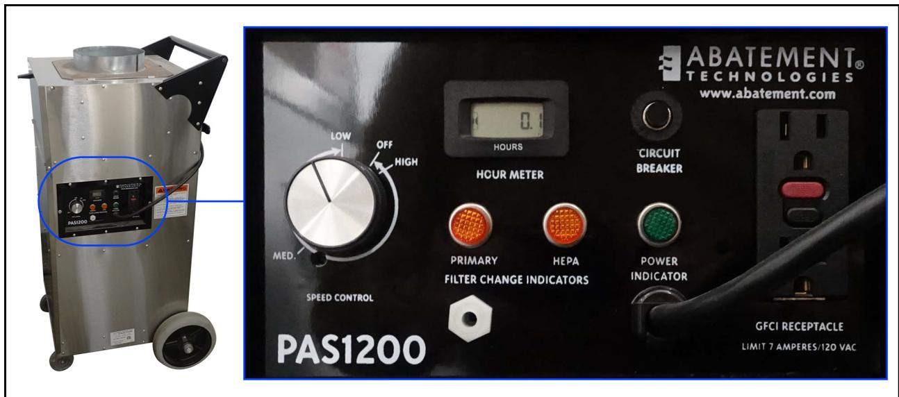
*Figure 6-7: Air Scrubber Unit with Control Panel*
