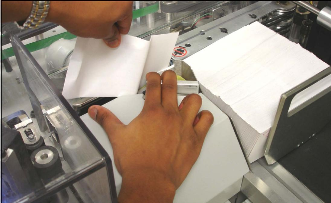
***Figure 3-24: Clearing envelope feeder jams***
