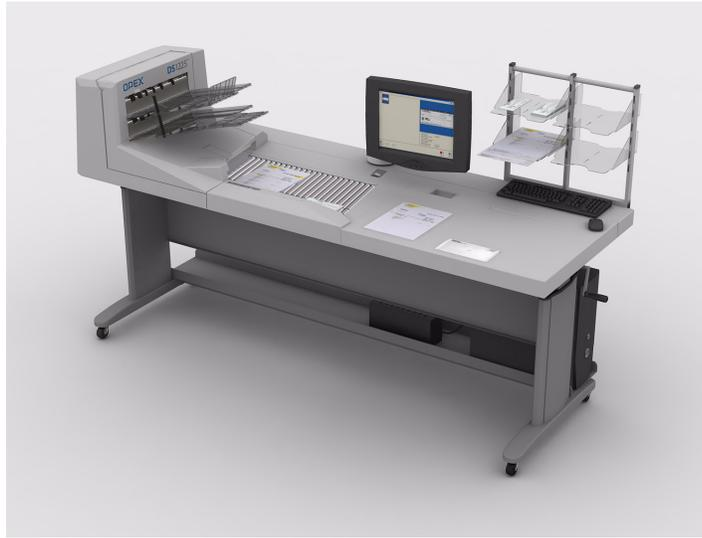
There is an optional, integrated workstation designed specifically for the DS1225. The optional table assembly is designed to convert the DS1225 into an integrated workstation. The height of the workstation can be adjusted from a minimum of 25 inches to a maximum of 36 inches via a hand crank. Locking front casters keep the unit stationary.
