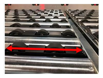
Figure 3-25: Containers move right or left when wheels are higher
