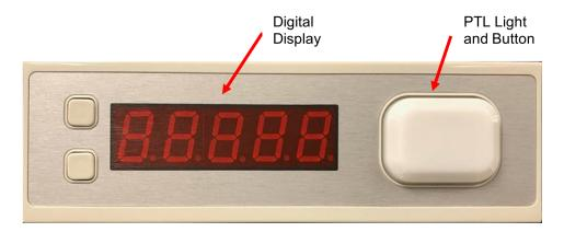
Figure 3-12: PTL unit above container on workstation
