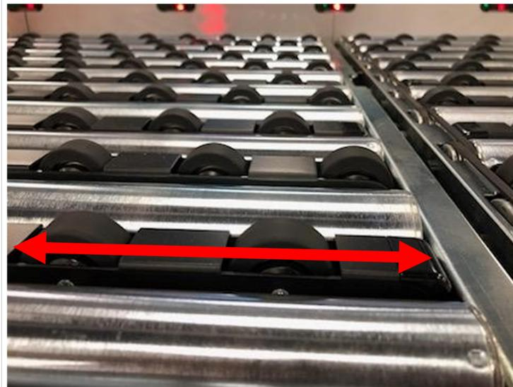
**Figure 3-25: Containers move right or left when wheels are higher**
