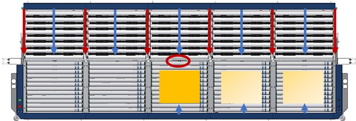
**Figure 3-31: Container moves to front, blocks only front stage sensor**
