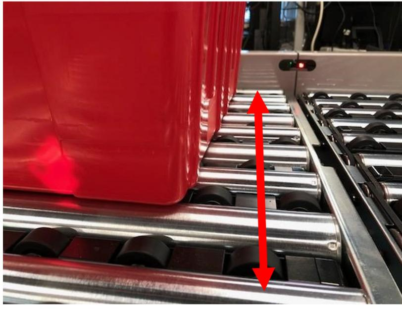
Figure 3-26: Containers move front or back when rollers are higher
