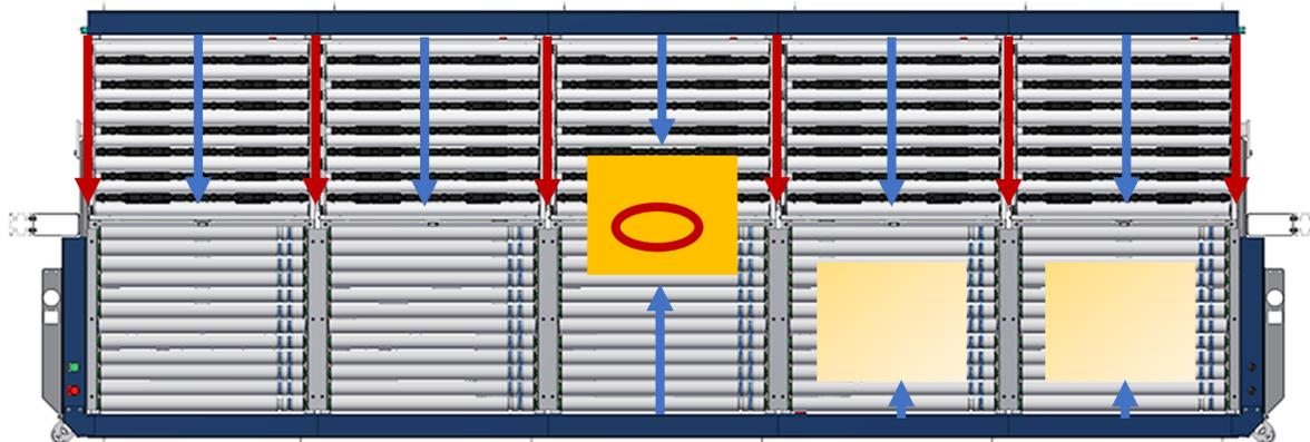
Figure 3-30: Container moves to front, blocks stage sensor and entry (center) sensor
