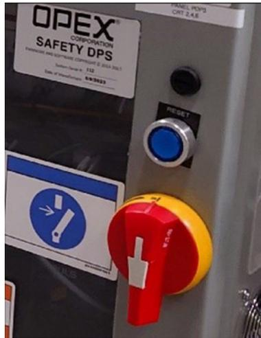
**Figure 5-54: Safety DPS unit with blue Reset button**
