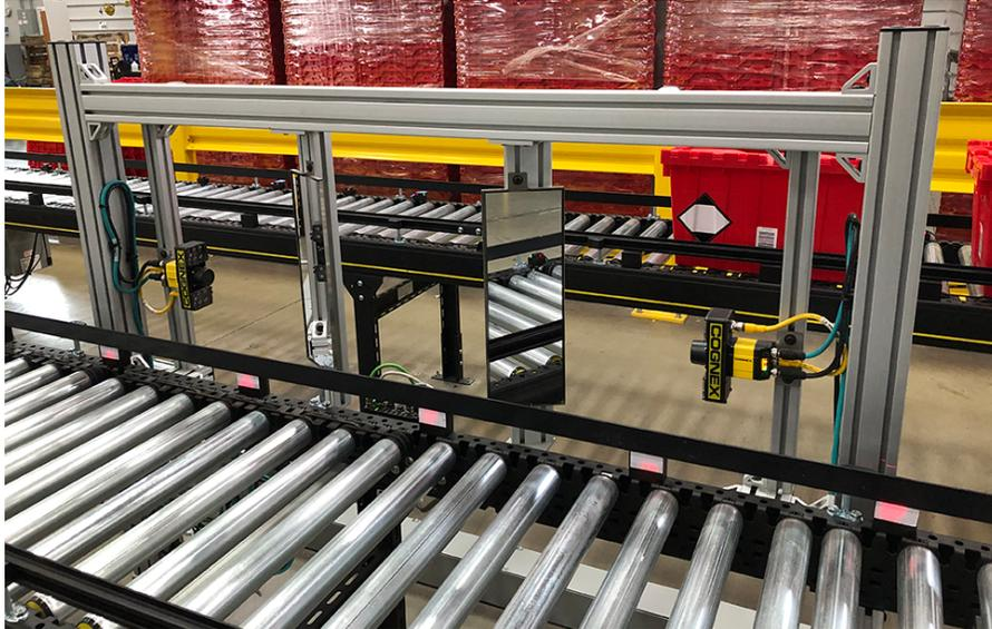
Figure 3-32: Scan tunnel
