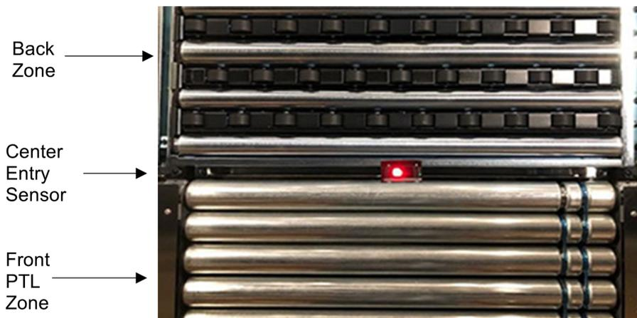
Figure 3-23: Close up view of entry (center) sensor
