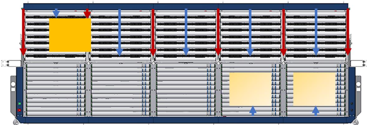
**Figure 3-29: Container exits, blocks stage sensor and second entry sensor**
