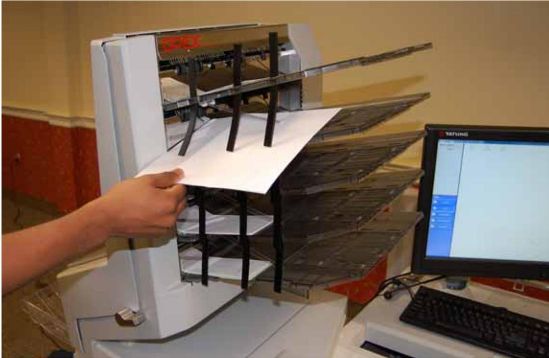
**Figure 22: Clearing the output bins**
