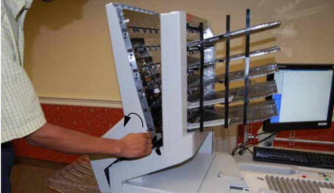
**Figure 21: Opening the stacker transport cover**
