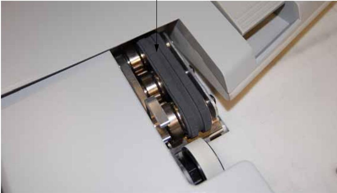
Lift the tab on the top of the feed assembly to clean the retard pad underneath. Also clean the feed rollers that lead up to the feeder.
