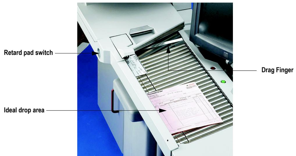
Since the feeder pulls from the top of the stack, the lead sheet in the stack must be the first to reach the feeder. If the bottom piece reaches the feeder first, a paper misfeed is likely to occur. There are techniques for learning to drop packets of paper consistently and effectively. The documents do not have to be perfectly
